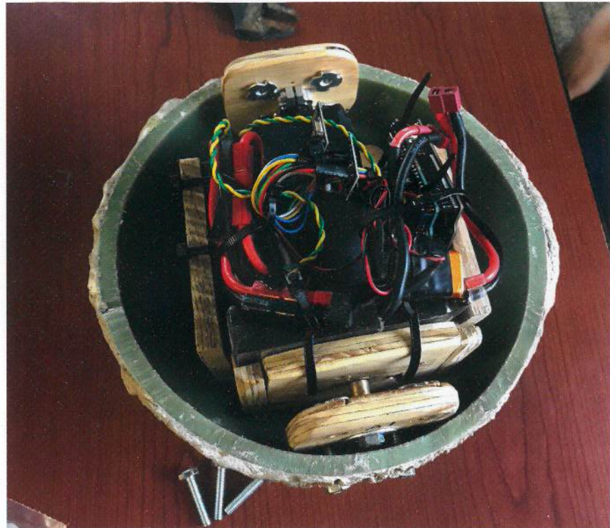
The cheetah ball's original design started with cutting the ball in half and mounting a motor and axel down the middle
